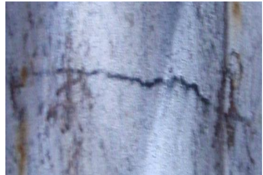
Image 2: screw 2 Etched cross section of the thread section in image 1 with incipient cracks
